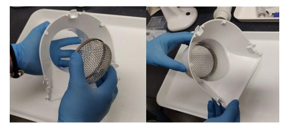
(2) Attach shield to funnel (Multiple can be setup prior to appointments). Attach onto middle tab first, then do the side tabs.
