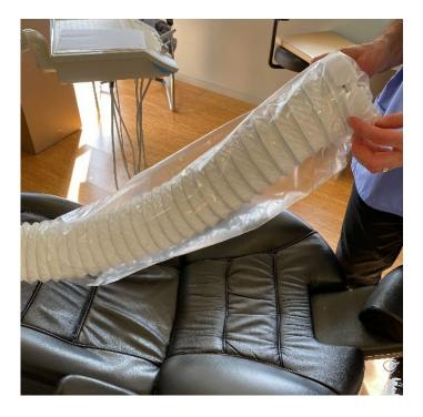
(4) Press and twist the tapered funnel end into the collar.
