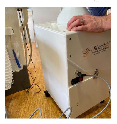
(4) Undo the side clips and slide the bottom section off.
