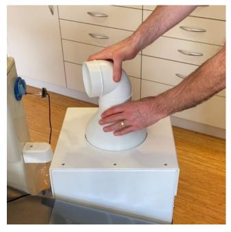
(5) Extend the 100mm duct(collar end) to the dental chair headrest and back to the 100mm elbow.
